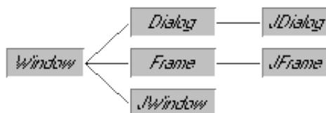
As the diagram shows, they all subclass window, not JComponent. This means they are not *lightweight*, have a peer, and cannot be transparent.
